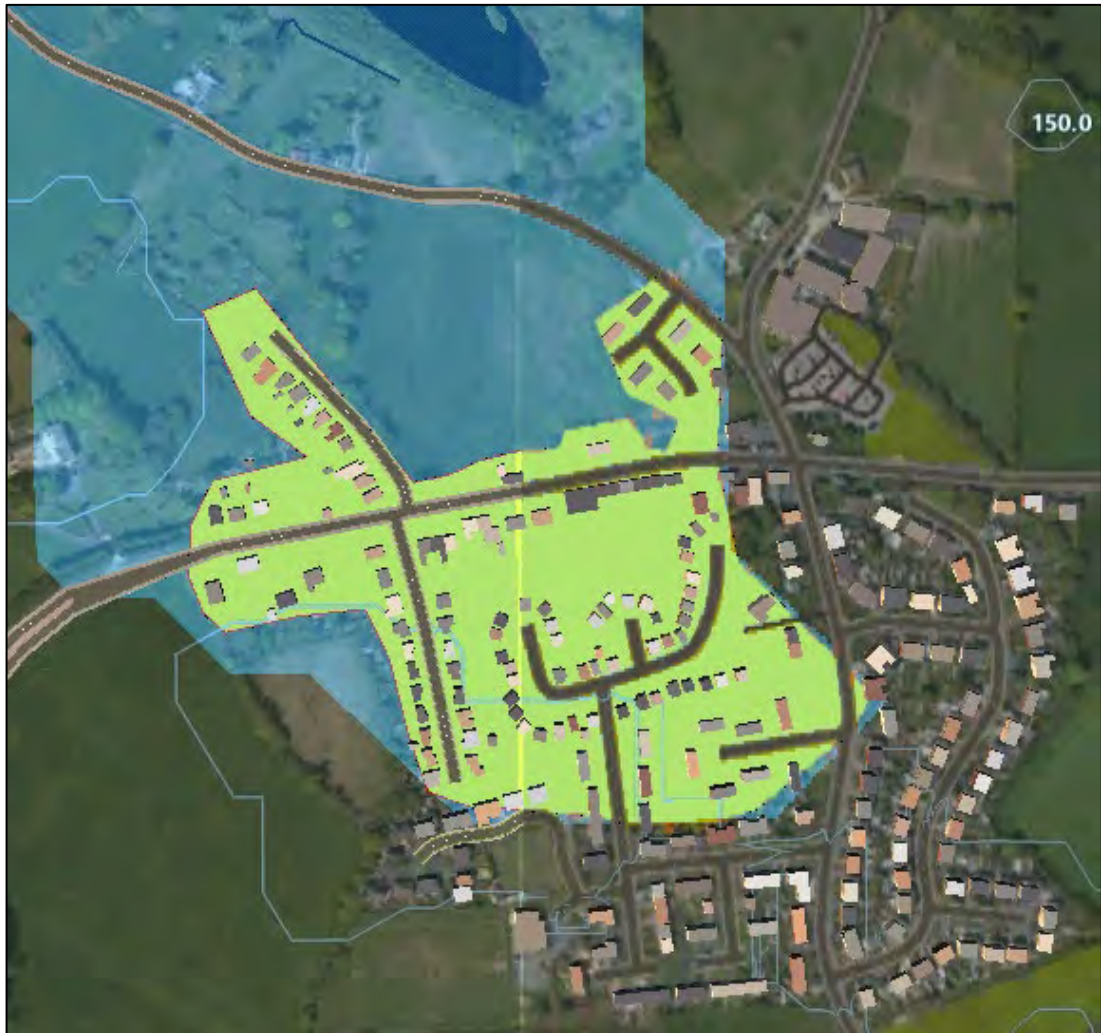
Figure 3: Upstream Catchment Contributing to Surface Water Flooding.
